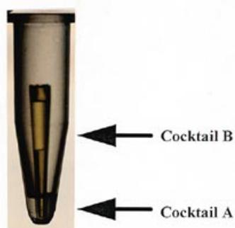
**Figure 1.** Simple and reliable device compartmentalizing an Eppendorf tube that allows capture, reverse transcription and nested-PCR in a single closed tube. Cocktail A corresponding to the reverse transcription and first PCR reaction mix is added to the bottom of the tube. Cocktail B, the PCR reaction mix for the second amplification, is added into the pipette tip cone.
