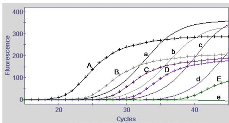
Fig. 6. A multiplex real-time PCR of serial dilutions ( $10^{-1}$ – $10^{-4}$ ) of DNA sample #988, from a field-grown, HLB symptomatic sweet orange tree from São Paulo, Brazil. Fluorescence data from channel 1 (plain lines a, b, c, d and e) for detection of the target DNA of *Ca. L. americanus* with the primer–probe set HLBampr and from channel 3 (asterisk-marked lines, A, B, C, D and E) for assessment of the quality of DNA extract with the positive internal control primer–probe set COXfpr.
