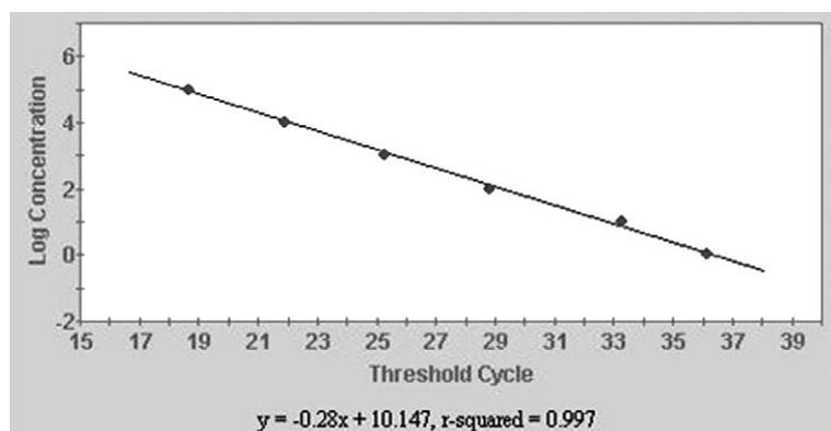
Fig. 3. A standard curve obtained in multiplex real-time PCR with primer–probe combinations HLBaspr and COXfpr using the serial dilutions (10<sup>0</sup>–10<sup>-6</sup>) of a DNA extract of a greenhouse-grown, HLB symptomatic, sweet orange plant inoculated with *Ca. L. asiaticus* strain B239.
