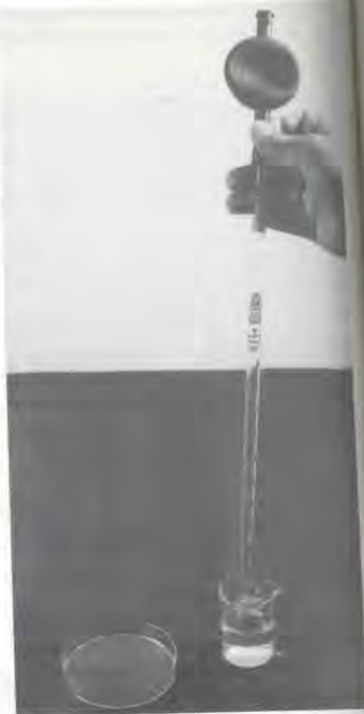
Fig. 21.3. Removal of top water with a pipette from the beaker. The remaining 15-20 ml water will be poured into the dish for final examination under stereoscopic microscope
