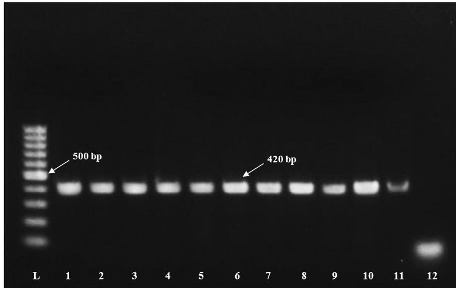
**Fig. 1.** PCR amplification of DNA from eight different *Heterodera* species with the universal actin gene primers (Hs-actF and Hs-actR) revealing a 420-bp fragment. Lanes: L = 100 bp DNA ladder (Fermentas Life Sciences); 1, 2 = *H. latipons* (Fa3); 3, 4 = *H. avenae* (Fa1); 5 = *H. hordecalis* (E69); 6, 7 = *H. filipjevi* (Did23b); 8 = *H. glycines* (HGRiggs); 9 = *H. schachtii* (HSPol); 10 = *H. betae* (DCP1248); 11 = *H. ciceri* (FaC3); 12 = Negative control. (See Table 1 for codes.)
