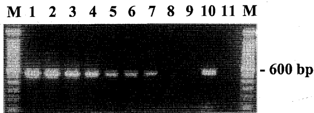
Fig. 2 Sensitivity of a PCR assay for detection of Ralstonia solanacearum in potato homogenate using primers PS-1/PS-2. Healthy potato tuber extracts were mixed with 10-fold dilutions of R. solanacearum cells. Lanes 1–8, dilutions of R. solanacearum cells ranging from 1 \times 10^6 to 0.1 CFU per PCR reaction mixture; lane 9, healthy potato sample; lane 10, genomic DNA of R. solanacearum (GSPB 1958); lane 11, negative control; lanes M, DNA size marker (100 bp ladder, Life Technologies)
