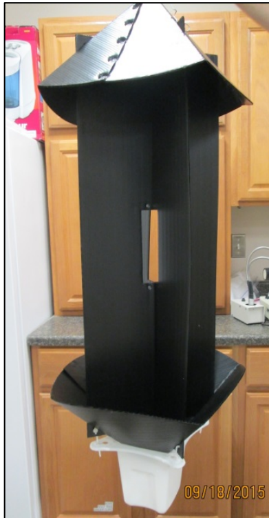
Figures 1 & 2. Cross Vane Panel Trap and collection cup.
