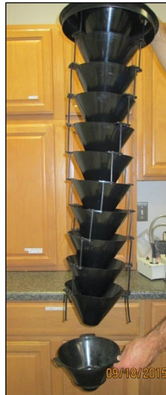
Figure 4. Bottom funnel of Multi-funnel Trap.
