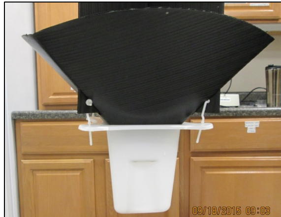
Figures 1 & 2. Cross Vane Panel Trap and collection cup.
