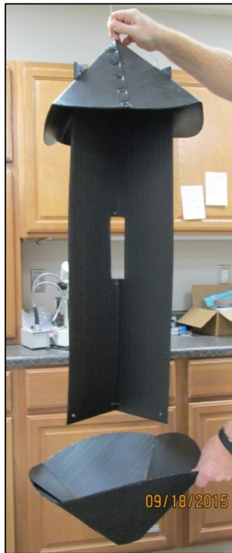
Figure 3. Bottom funnel of Cross Vane Panel Trap.
