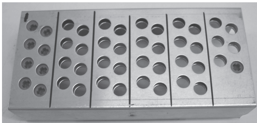
Fig. 1. Metal rack specially designed to hold 'MiniCollect tubes' so that stoppers are held in place while sampling contents of four tubes at a time. Stoppers of nine tubes are visible.
