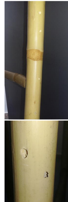
Fig. 2: Exit holes of C. annularis in dried bamboo furniture (Photo from Suma, P. & S. Bella, 2018)
