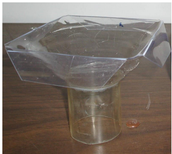
Figure 3. Internal funnel for Dendrolimus traps. (Image courtesy of David Lance, USDA-APHIS-PPQ.)
