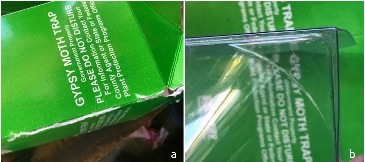
Figure 4. a. Milk carton trap with cracked and torn edges caused by inserting milk carton funnel insert. b. Squared corner of milk carton funnel insert. Images courtesy of Dale Anderson (South Dakota Dept. of Agriculture)
